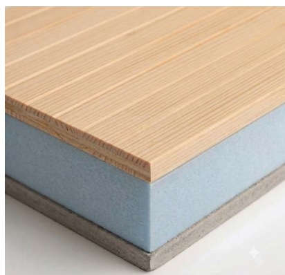
ThermoChip TAFbc/10-40-12 Tablero exterior cemento 12,5mm Núcleo XPS 40mm Tablero interior de friso 10mm
