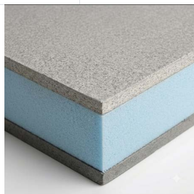
ThermoChip TYFbc/12-40-12 Tablero exterior cemento 12,5mm Núcleo XPS 40mm Tablero interior fibroyeso 12,5mm
