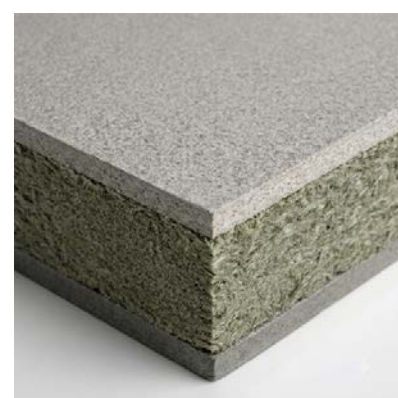
ThermoChip TYFbc(LR)/12-40-12 Tablero exterior cemento 12,5mm Núcleo LR 40mm Tablero interior fibroyeso 12,5mm
