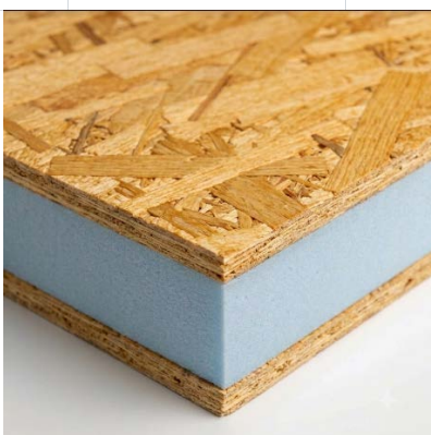
ThermoChip TOO/15-40-15 Tablero exterior de OSB 15mm Núcleo XPS 40mm Tablero interior de OSB 15mm
